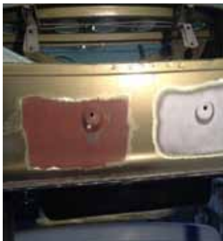
Paint stripping old-timer: Left, only with dry ice - Right, a combination of dry ice and an abrasive agent
